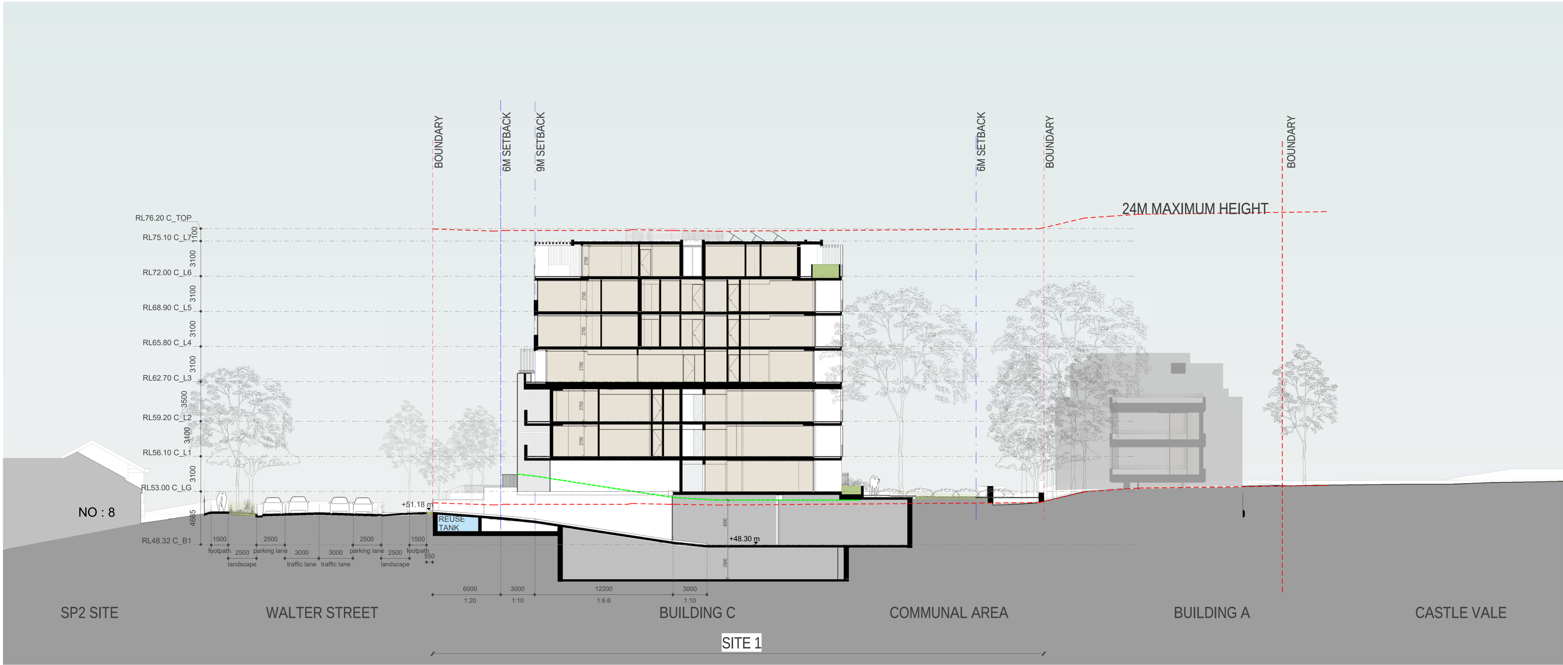
CROSS SECTION BLDG C DRIVE WAY 1 : 200
